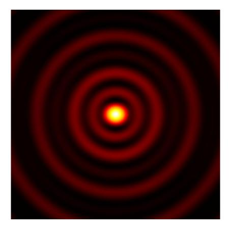
It is known that the vectorial nature of light plays a non-negligible role in high-NA focusing situations. In this example, focusing of a linearly polarized Gaussian beam by a high-NA aspheric lens is presented, and the asymmetric PSF in the focal plane is shown. By examining the electromagnetic field components in the focal plane, it can be found that the asymmetry is caused by a relatively strong  $E_z$  component.
